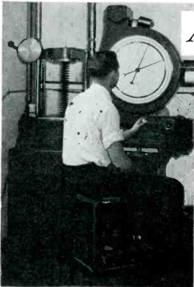
Conducting routine test on Olsen machine in Hunter's Inspection Department
