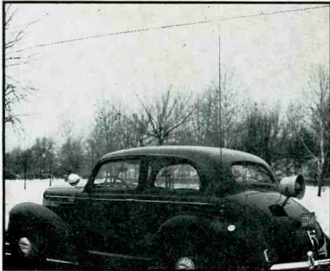
Fig. 4—Line supervisor's radio-equipped car. The loudspeaker at the rear is used to give orders to crews or to caution crowds
