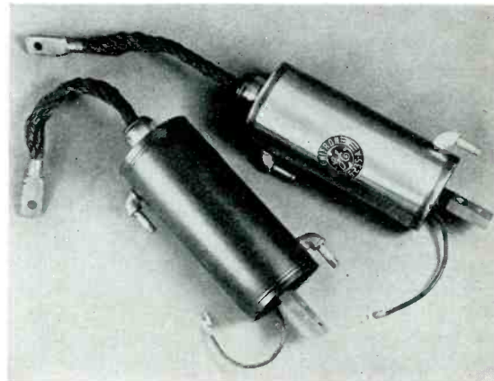
Two General Electric Company ignitron tubes (old and new styles) for welding control. These water-cooled mercury-pool controlled-rectifier tubes are particularly adapted to welder control service because of their ability to carry very high peak currents for short periods
